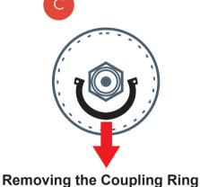
Remove the coupling ring to release the connection.
