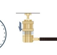
**Removing the Cap** Remove the cap from the female coupling on the hose. Ensure the cap is fully retracted to allow proper coupling.
