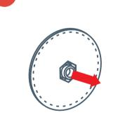
**Inserting the Coupling** into the Washer Insert the male coupling into the washer. Confirm proper placement before proceeding to the next step.
