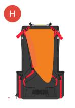
**Bag Removal** Remove the damaged or empty bag from the back of the backpack.
