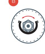
**Opening the Safety Ring** Open the safety ring that secures the coupling.
