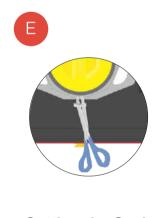
**Cutting the Seal** Cut the seal securing the filling mouth, allowing the inner bag to be released.
