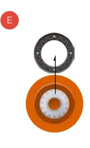
Fit the ribbed area of the discharge mouth with the ribbed area of the lower washer of the backpack.
