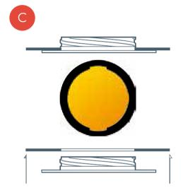
Align the recesses of the backpack washer with the bag.
